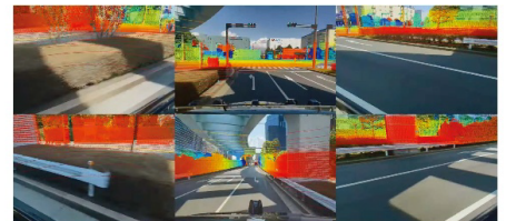
Camera/LiDAR sensor temporal alignment
