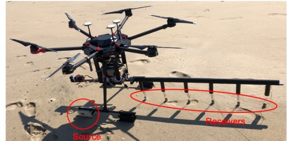
Six receivers and one source in a ~1.5 m array.
