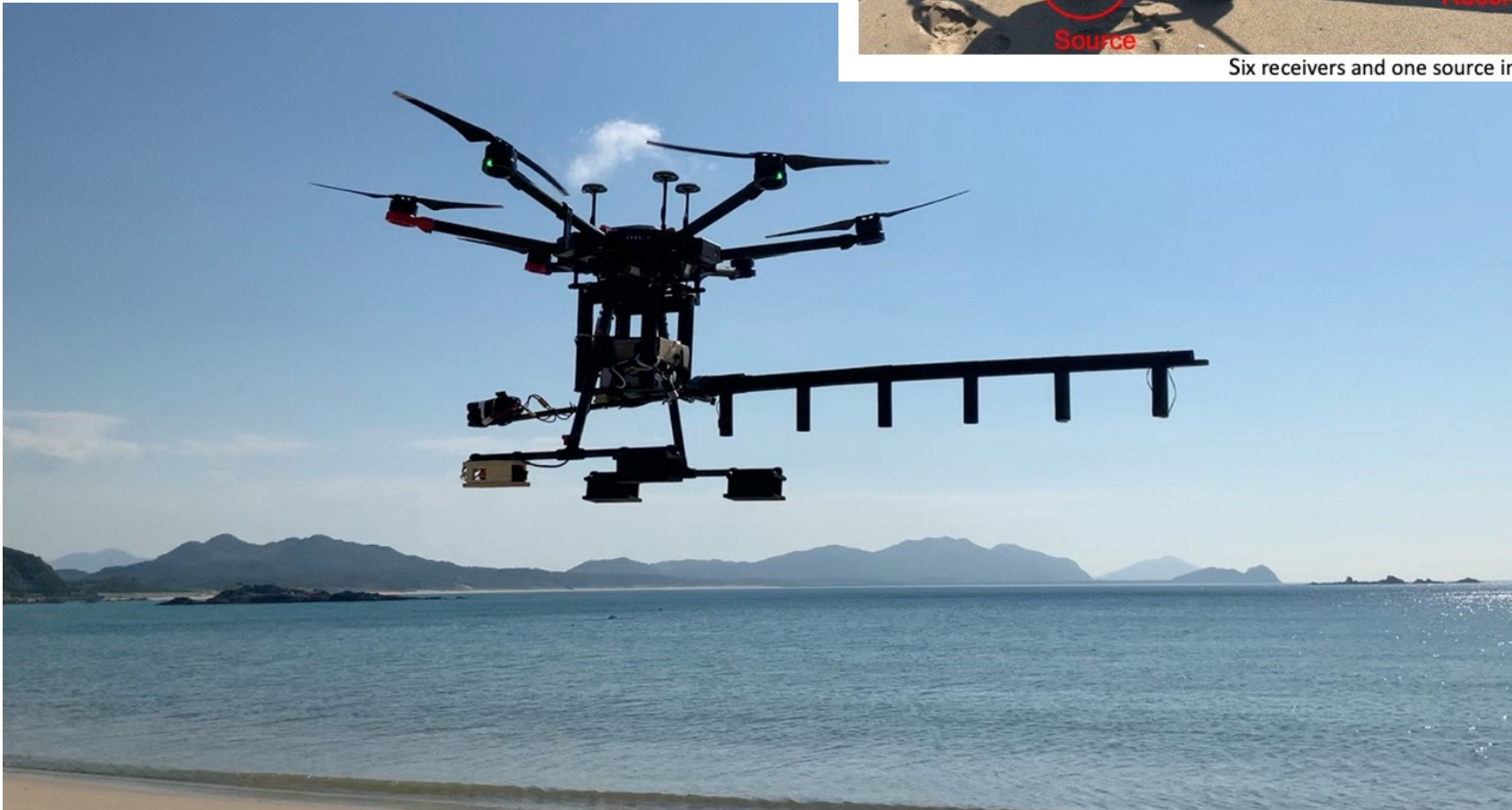
Six receivers and one source in a ~1.5 m array.
