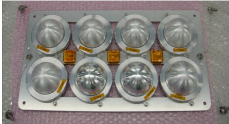
Shielding case with varying thickness (0.3 – 4mm, Al)
