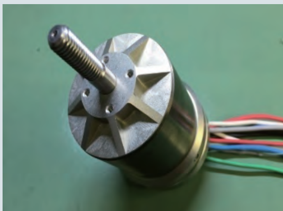
Primary prototype of IP56 clear dustproof and waterproof motor
