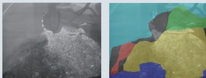
Fig. 4. Examples of image recognition using AI deep learning Left: Original image (during simulated rock excavation) Right: Region identification (yellow: excavated gravel, green: tunnel cross-section)
