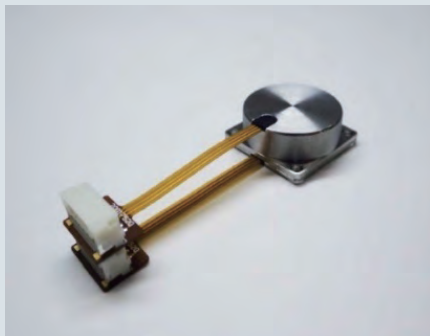
Ultra-small sensor for absolute angles Outer dimensions of product : Square 20 mm and thickness 7.5 mm Resolution 1048576
