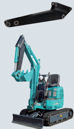
Carbon fiber (CFRP) stick installed in a hydraulic excavator (actual)
