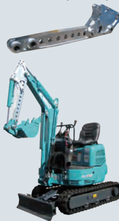
Lightweight metal stick installed in a hydraulic excavator (actual)
